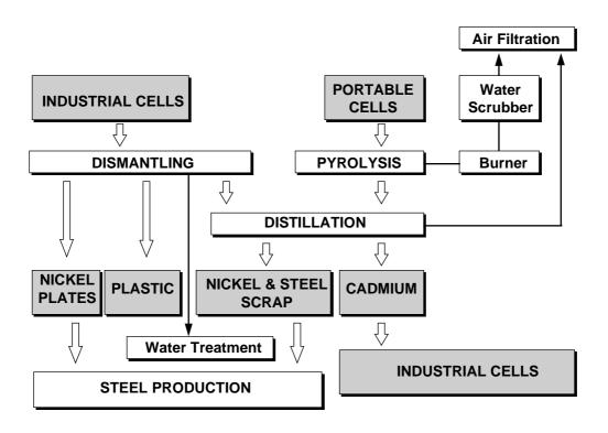
Figure 2: SAFT Recycling of Ni-Cd Btteries
