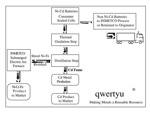
Flow Sheet 2: Processing of Consumer Ni-Cd Batteries
