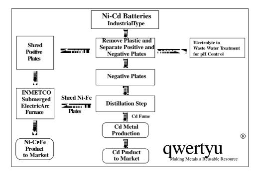
Flow Sheet 1: Processing of Industrial Ni-Cd Batteries
