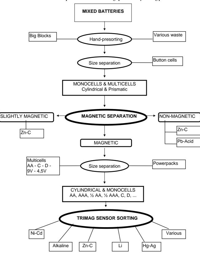
Graph I: Flow chart showing spent battery sorting process
