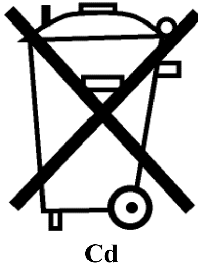
Figure 15. NiCd Battery Labeling Requirement of 91/157/EEC and 93/86/EEC
